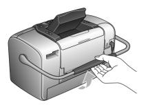
5. Open the cartridge compartment cover on the back of the printer.
